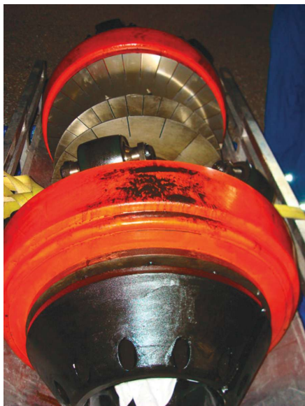
A cleaning pig appears clean in the receiving barrel with only a small amount of sand on the rubber. Photo courtesy of Jenny Been, TransCanada Pipelines.
